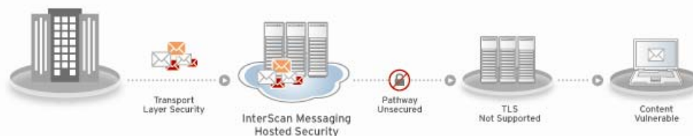
Figure 1: TLS only protects a portion of the path along which the data travels and may not be supported along the complete pathway.
